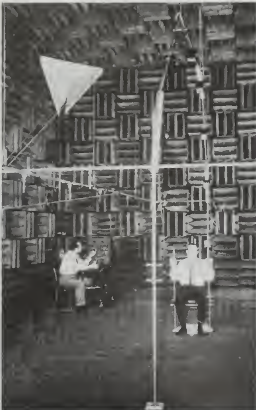
Auditory localization experiment in an anechoic chamber
